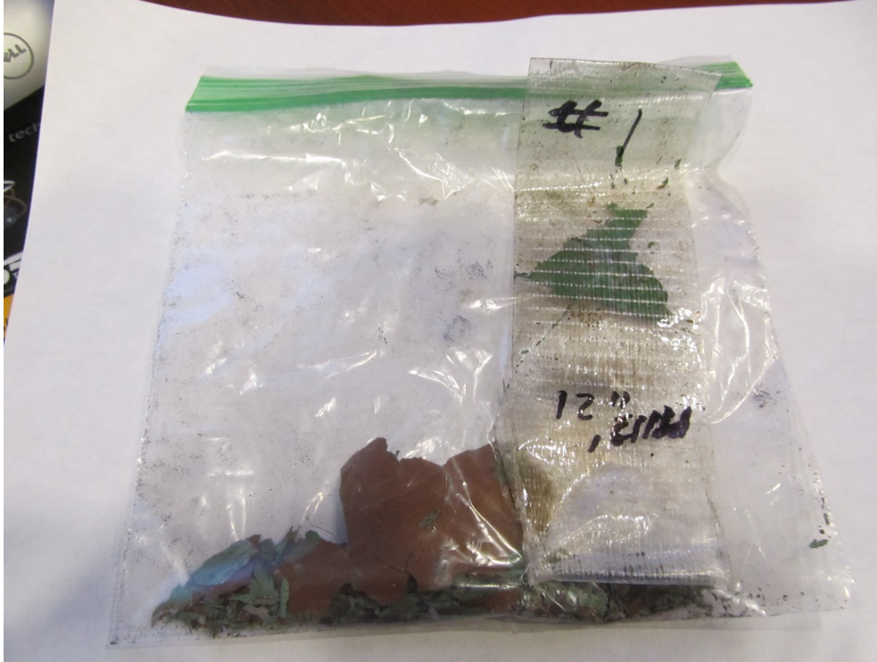
28) Adhesion test results and lab sample scrapings. All coatings were poorly adhered.
