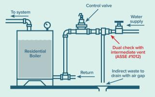
Boilers with chemical additives require an ASSE #1013 – Reduced Pressure Principle Backflow Prevention Assembly.
