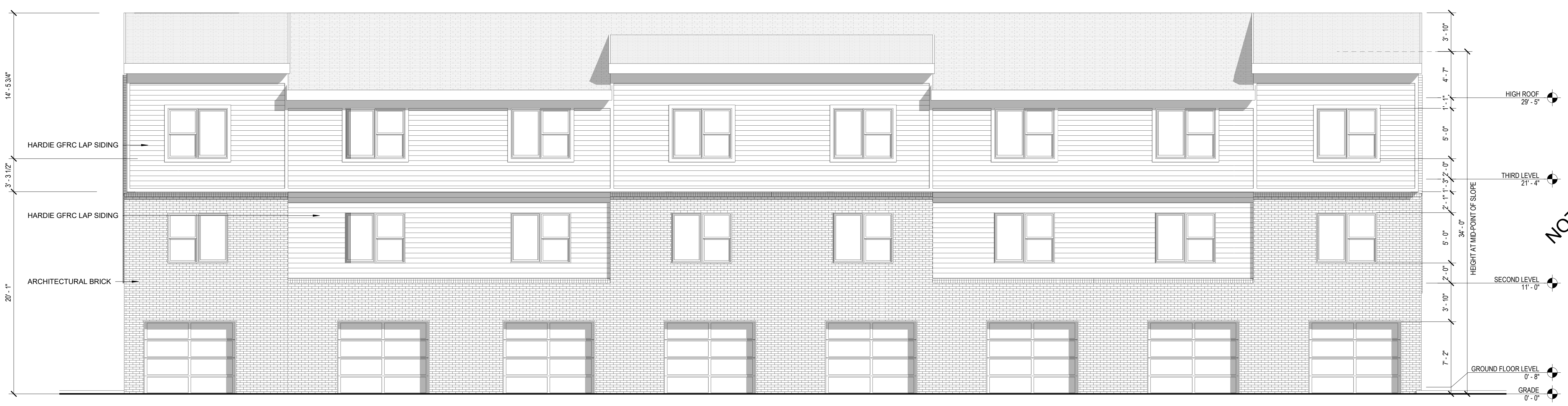
1 EIGHT-UNIT BUILDING - REAR ELEVATION SCALE: 3/16" = 1'-0"
