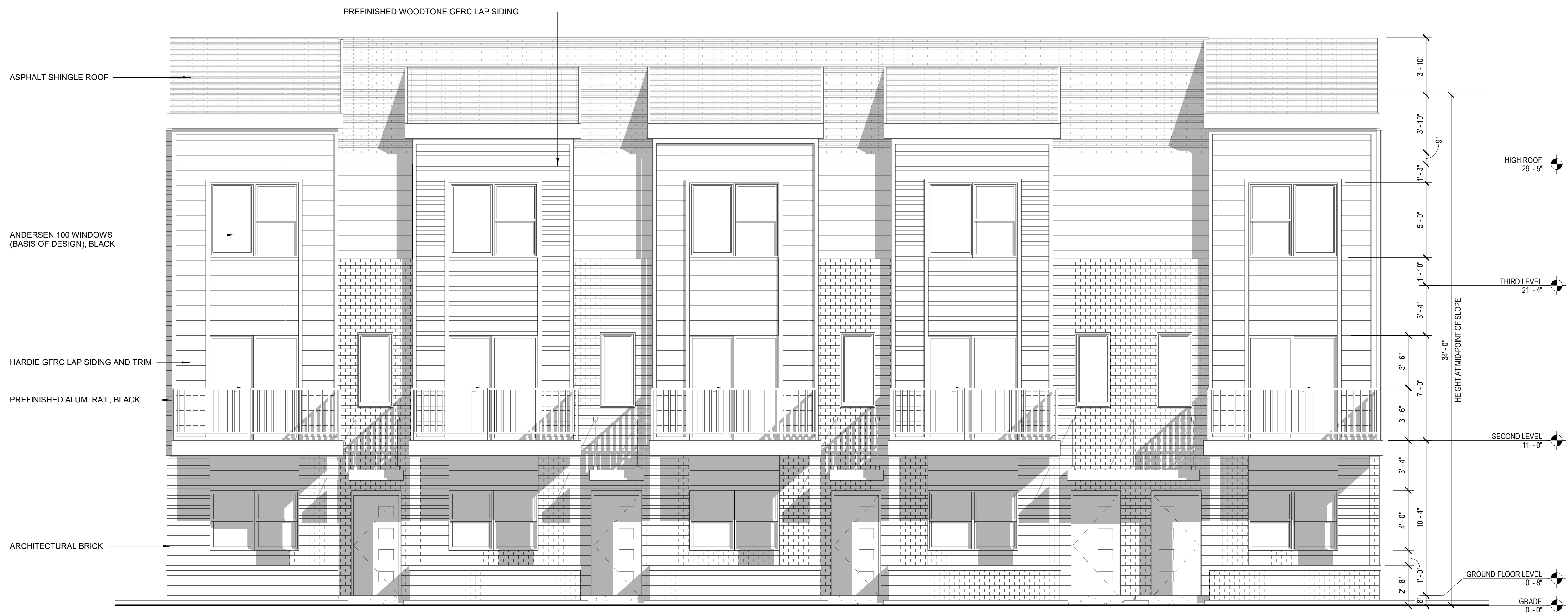
1 FIVE-UNIT BUILDING - FRONT ELEVATION SCALE: 1/4" = 1'-0"
