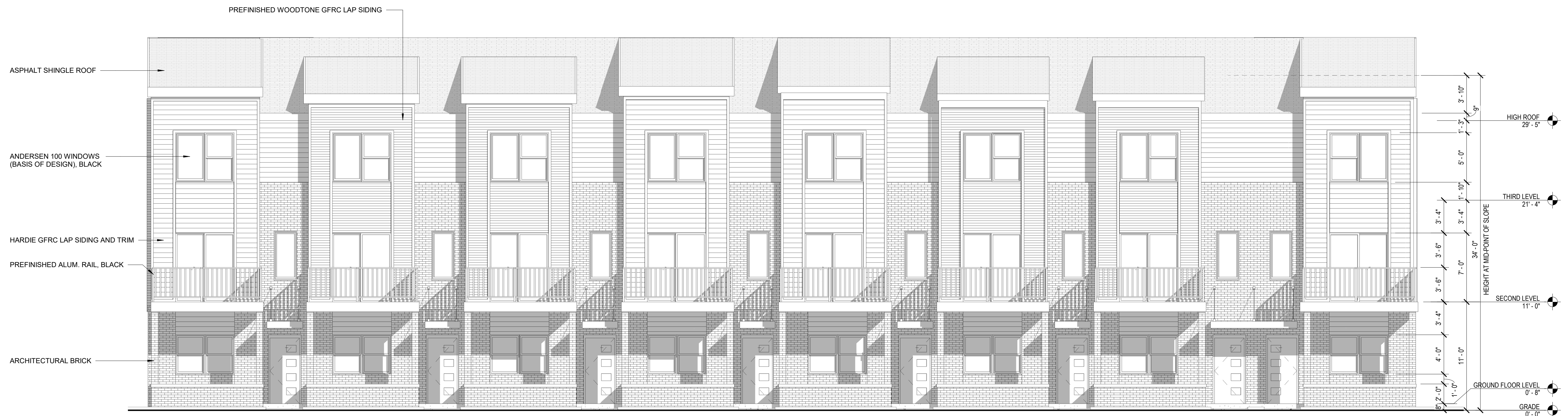
2 EIGHT-UNIT BUILDING - FRONT ELEVATION SCALE: 3/16" = 1'-0"
