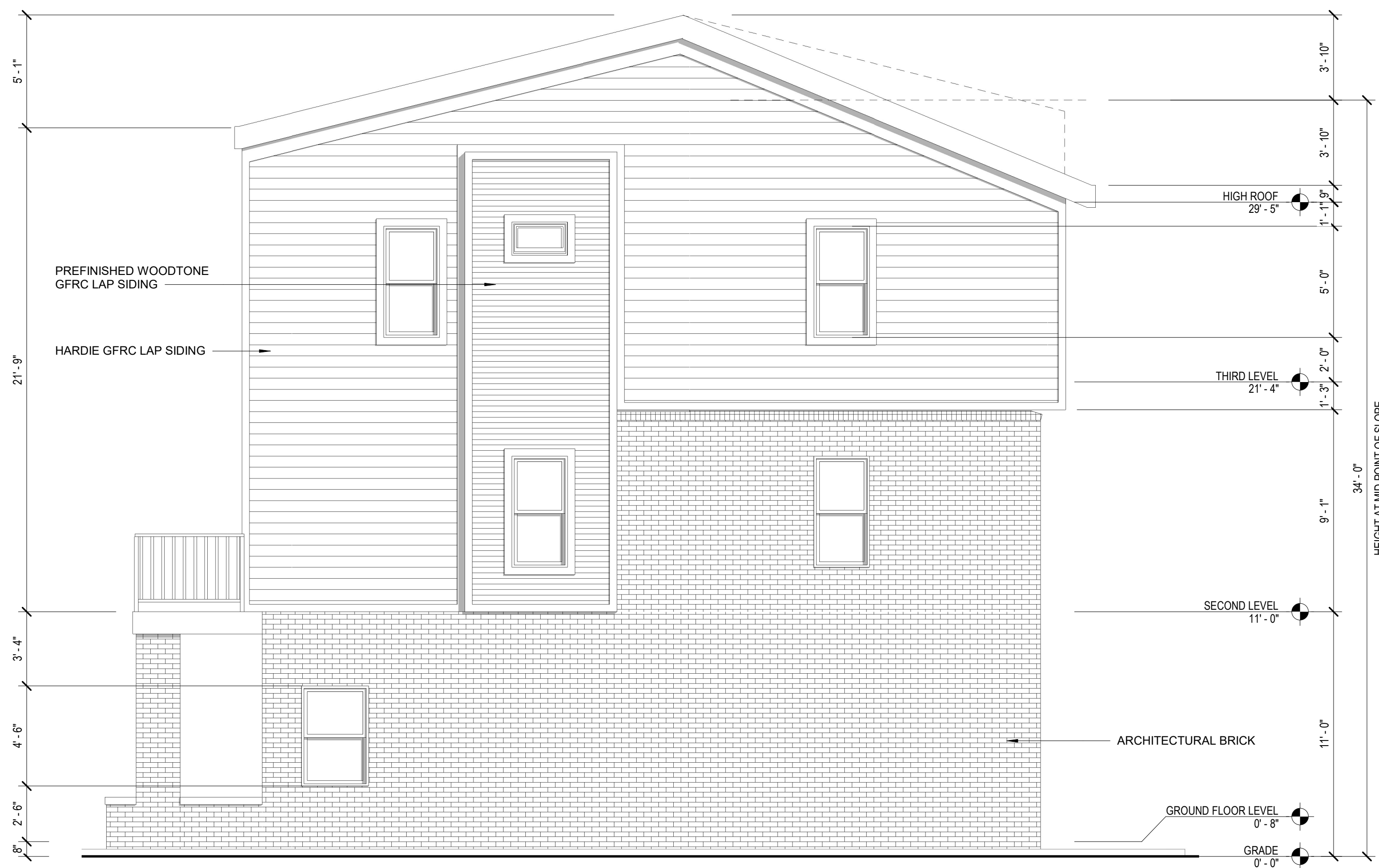
2 TYPICAL SIDE ELEVATION SCALE: 1/4" = 1'-0"
