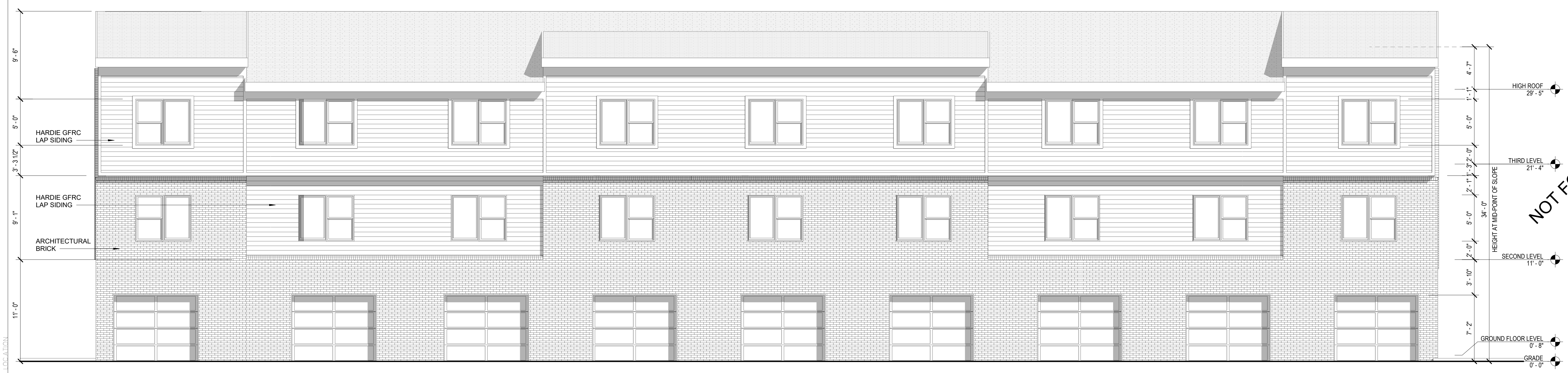
1 NINE-UNIT BUILDING - REAR ELEVATION SCALE: 3/16" = 1'-0"
